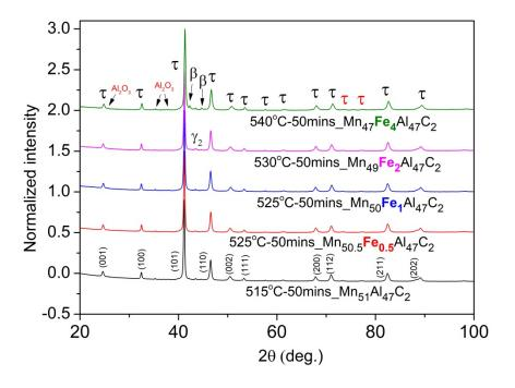
Figure 5. XRD diagrams of aged Mn(Fe)AlC alloys.
