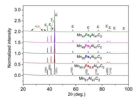
Figure 3. XRD diagrams of annealed Mn(Fe)AlC alloys.
