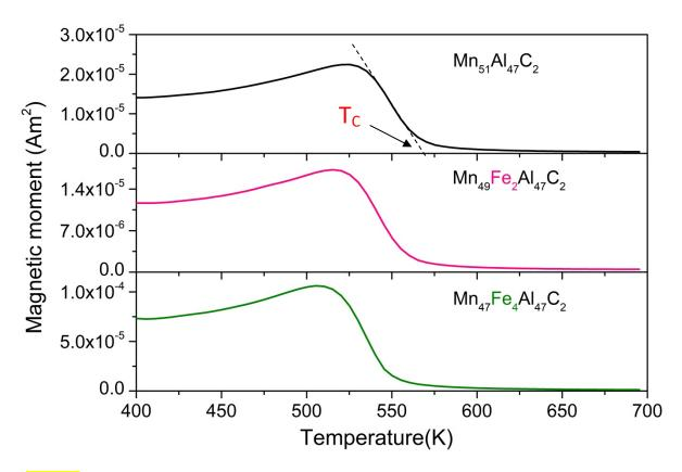
Figure 11. M-T curves on heating and cooling of aged Mn51Al47C2, aged Mn49Fe2Al47C2, and aged Mn47Fe4Al47C2.
