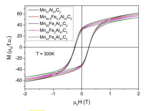
Figure 7. Hysteresis of aged Mn(Fe)AlC ferromagnetic alloys
