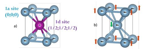
**Figure 1.** (a) Ideal equiatomic  $\tau$ -Mn<sub>50</sub>Al<sub>50</sub>, b)  $\tau$ -phase is obtained with an excess of Mn at 1d site (1/2;1/2;1/2) ( about 4 at.%) showing the antiferromagnetic coupling between Mn atoms at 1a and 1d sites.
