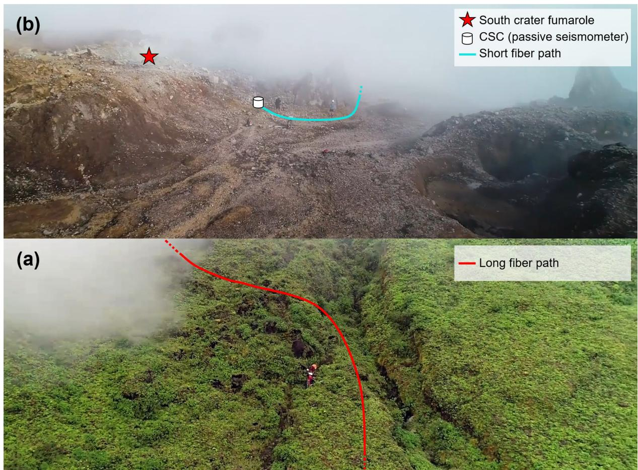
Figure 4: (a) Summit area of the volcano, bare of vegetation due to the acidic environment. Seismometer is under the smoke plume of the fumarole. (b) Long fiber installation along the luxuriant flank of La Soufrière Volcano. The team is moving along the path (center), laying the cable on the vegetation.
