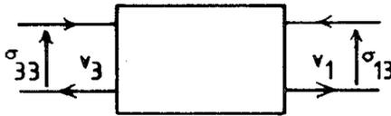
FIG. 2. A layer of elastic material bonded onto a rigid backing, in a plane acoustic field, and the equivalent electrical system related to stress and velocity components at A.
