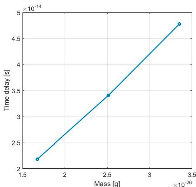
**Figure 4.** The mass sensitivity of the IIP/SAW device.
