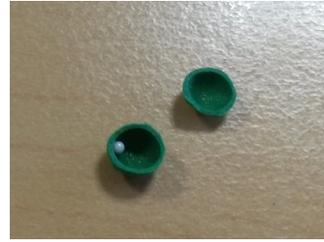
**Fig. 13** Viscoelastic hollow grains (ref. E171101, ATECA, France).
