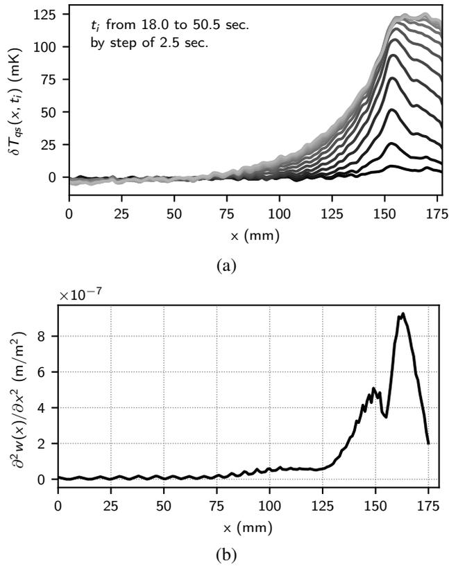
FIG. 11. (a) Measured  $\delta T_{qs}(x, t_i)$  for  $t_i$  ranging from (black) 18.0 sec. to (light grey) 50.5 sec. with time steps of 2.5 sec., and (b) estimated  $\partial^2 w(x)/\partial x^2$  at 933 Hz.
