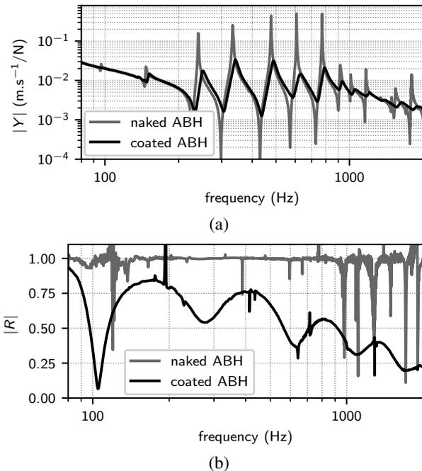
FIG. 2. (a) Magnitude of the mobility of the excitation point ( $x = -500$  mm); (b) modulus of the reflection coefficient of the (black) coated and (gray) naked ABH calculated at  $x = 0$ . A 50 mm-wide grid of  $26 \times 6$  measurement points located in the region  $x < -125$  mm is used in order to verify the far-field conditions.
