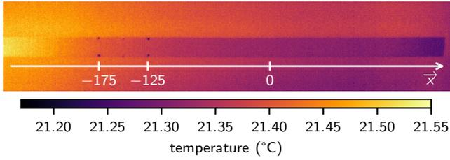
FIG. 5. Example of thermogram of the beam at rest, averaged in time over 30 thermograms (15 sec.), used to measure  $T_0(x)$ .
