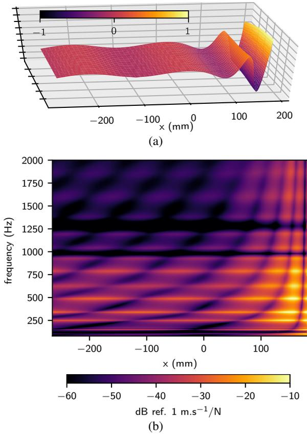
FIG. 3. (a) Snapshot of the measured velocity of the coated ABH at 1,000 Hz; the ABH begins at  $x = 0$  and the amplitude is normalised to its maximum value; (b) absolute value of the frequency response functions  $Y(\omega, x) = V(\omega, x)/F(\omega)$  where  $V(\omega, x)$  is the velocity spectrum, at point  $x$  belonging to the bottom end of the coated ABH, and where  $F(\omega)$  is the applied force spectrum at the driving point.
