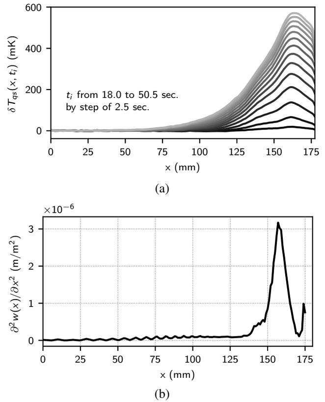
FIG. 10. (a) Measured  $\delta T_{qs}(x, t_i)$  for  $t_i$  ranging from (black) 18.0 sec. to (light grey) 50.5 sec. with time steps of 2.5 sec., and (b) estimated  $\partial^2 w(x)/\partial x^2$  at 276 Hz.
