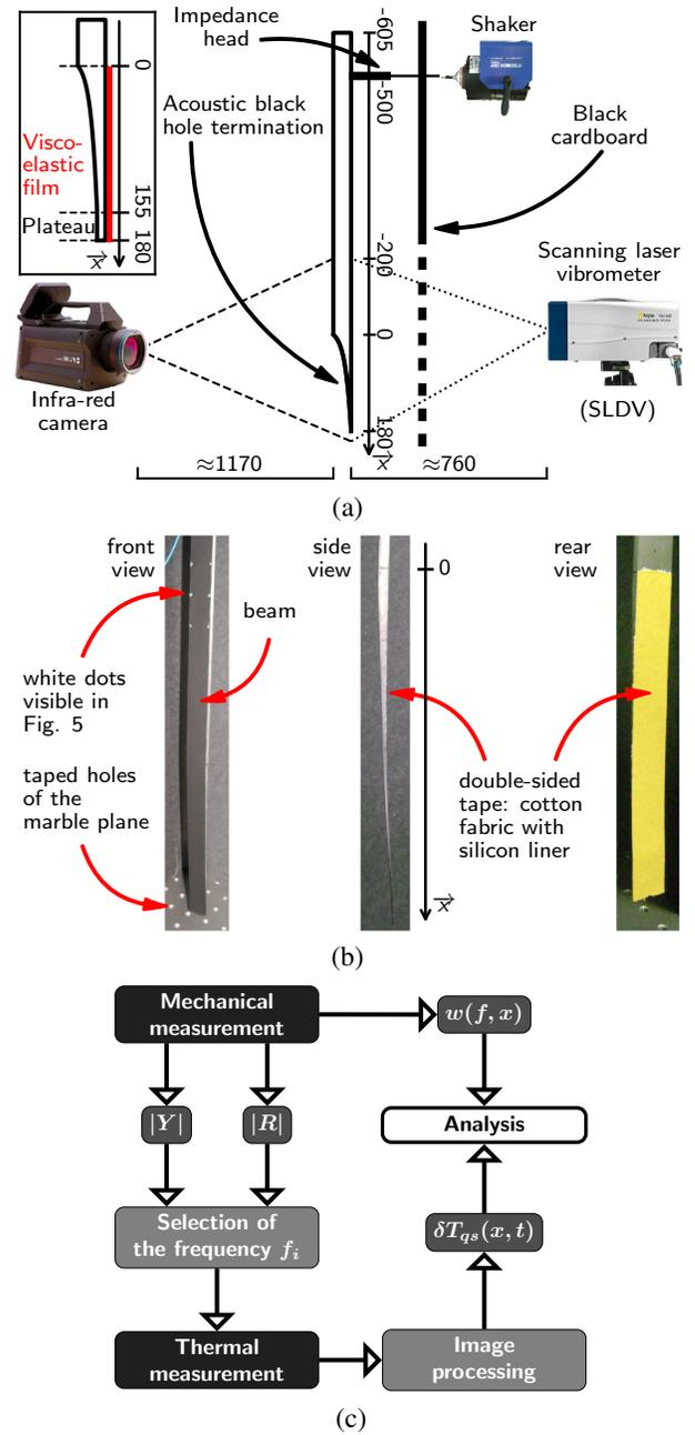
FIG. 1. (a) Sketch of the experimental set-up, with dimensions expressed in mm (ABH begins at  $x = 0$ ); (b) pictures of the ABH (covered with visco-elastic material), front, side and rear views; the front (measured) side is painted black; the profile of the ABH is visible on the side view; the rear view shows the ABH with the visco-elastic film; (c) block diagram of the proposed method.
