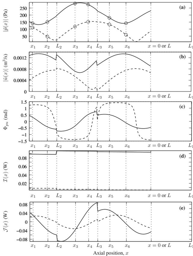
FIG. 3. Spatial distribution of the acoustic field with respect to the  $x$ -coordinate: (a) modulus  $|\bar{p}(x)|$  of the acoustic pressure, (b) modulus  $|\bar{u}(x)|$  of the acoustic volume velocity, (c) phase shift  $\Phi_{pu}(x)$  between acoustic pressure and acoustic volume velocity, (d) active acoustic power  $\mathcal{I}(x)$ , and (e) reactive acoustic power  $\mathcal{J}(x)$ . The open circles correspond to the measured acoustic pressures  $\bar{p}(x_i)$ .
