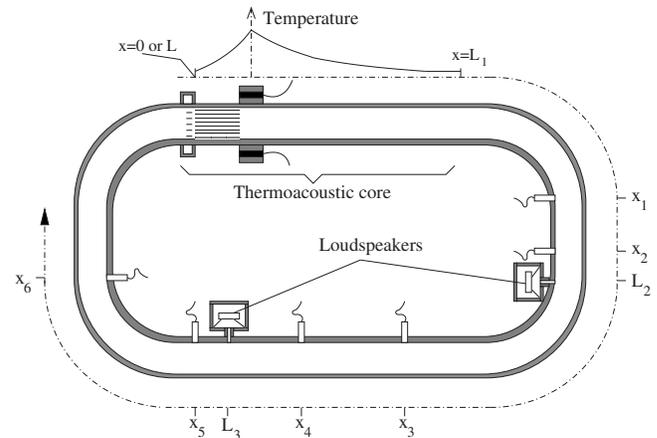
FIG. 1. Schematic diagram of the experimental apparatus. The spatial positions of the six microphones are  $x_1=0.575$  m,  $x_2=0.764$  m,  $x_3=1.162$  m,  $x_4=1.344$  m,  $x_5=1.612$  m,  $x_6=1.866$  m, and the positions of the auxiliary sources are  $L_2=0.91$  m and  $L_3=1.47$  m.
