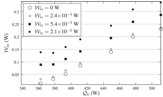
FIG. 4. Acoustic power  $\mathcal{W}_{ac}$  available in the cold part of the waveguide with respect to the heating power supply  $\mathcal{Q}_h$  for different electrical powers  $\mathcal{W}_{ls}$  provided to the loudspeakers.
