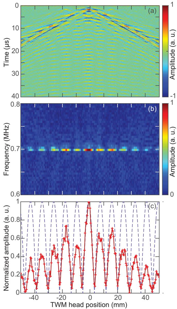
Figure 4: (color online) The thermoelastic source is a line  $4.1 \times 20 \text{ mm}^2$ : (a) time domain and (b) frequency domain B-scans as a function of the TWM head position. (c) First ZGV peak amplitude vs. TWM head position: experimental (solid) and theoretical (dashed) curves.
