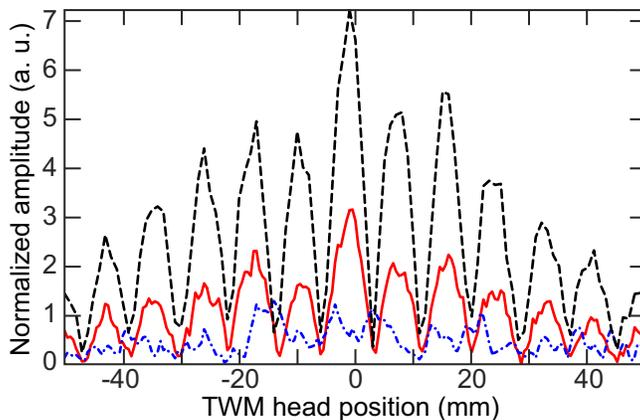
Figure 5: (color online) Normalized first ZGV peak amplitude vs. TWM head position when the thermoelastic source is a single line (solid), multiple lines spaced by  $\lambda_{ZGV}^{Al}$  (dashed) and multiple lines spaced by  $\lambda_{ZGV}^{Al}/2$  (dash-dotted).
