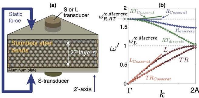
FIG. 1 (color online). (a) Experimental setup. (b) Theoretical dispersion curves for propagation in the *z* direction of the hcp granular crystal from the discrete lattice model (circles) and their counterparts from the Cosserat continuum model (lines). The cyclic frequency is normalized to the cutoff cyclic frequency  $\omega' = \omega/\omega_L^{c,discrete}$  of the mode *L*.
