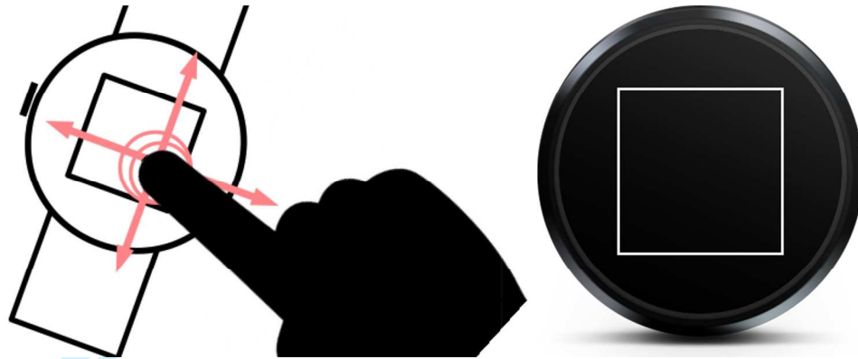
Figure 7. Swipe/Tap patterns (left) and real ControlWear "TrackPad mode" screenshot (right)
