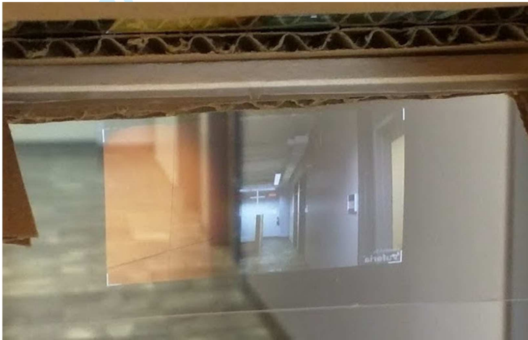
40 Figure 10. View of the camera’s phone projected to the plastic sheet of CARTON
